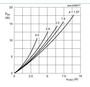
$\begin{array}{l} \textbf{a} = form \ factor = I_{F(RMS)} / I_{F(AV)} \\ Vo = 1.268 \ V; \ Rs = 0.031 \ \Omega \\ \hline \textbf{Fig. 2. Forward power dissipation as a function} \\ \textbf{of average forward current; sinusoidal waveform;} \\ \hline \textbf{maximum values} \end{array}$
