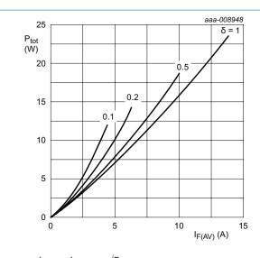
$\begin{array}{l} {\sf I}_{\sf F(AV)}={\sf I}_{\sf F(RMS)}\times\sqrt{\delta}\\ {\sf V}_{o}=1.268~V;~{\sf R}_{s}=0.031~\Omega\\ \end{array}$  Fig. 1. Forward power dissipation as a function of average forward current; square waveform; maximum values
